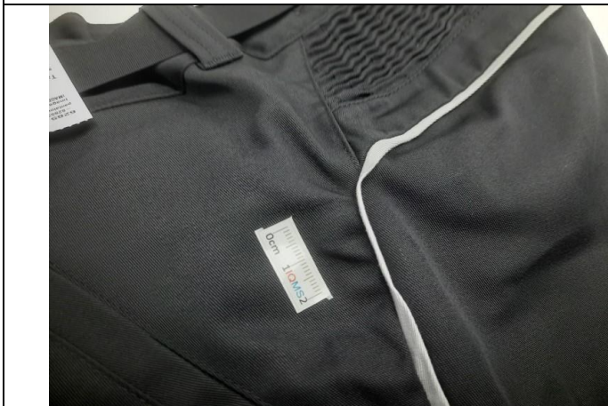
Seam puckering at side seam - Major
