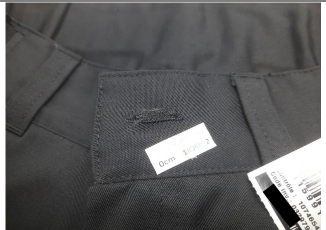
Unclean buttonhole - Minor
